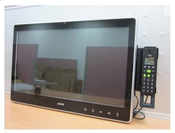
Step 1: Fasten the two screws(2-SELF TAPPING SCREWS) to fix the Skype Bracket with the ACP-5217
